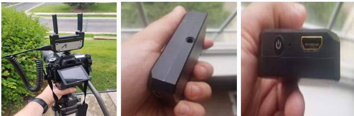
The physical design of the [CineEye](#) is nice and sleek. There is a single HDMI port, a power button, a USB-C port for charging, and a threaded mounting hole. It’s kind of all that you need on a smaller unit like this. There are also 4 LED indicator lights on the front panel to show the remaining battery.
