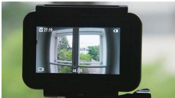
The image distortion can be repaired with the in-camera de-warp function.
